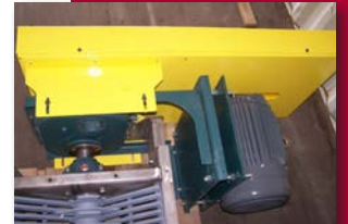
Lump Busters Feature Dodge Drive Components
